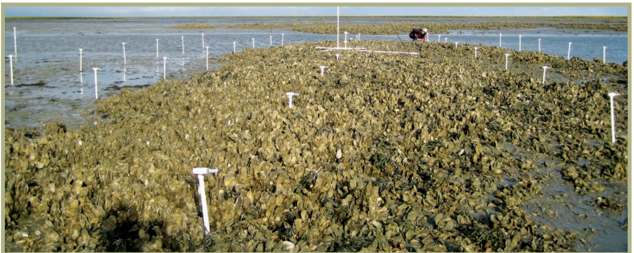
Figure 35. A reef with light sensors deployed. Note: The sensors depicted have been deployed in a grid pattern, not as described in the text.
